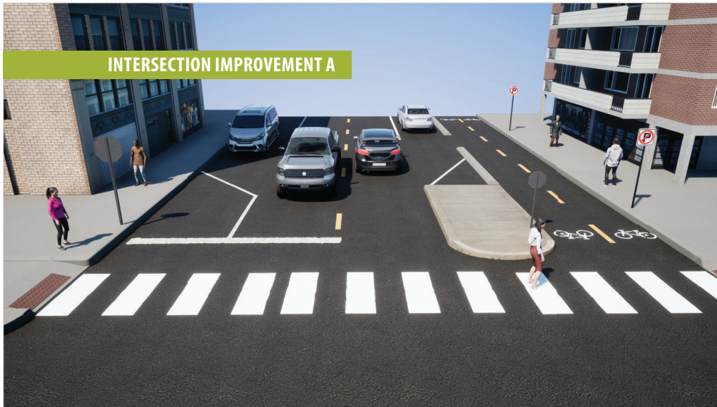
Intersection improvement A – parking lane safety island (5th Ave, Portland Ave, Chicago Ave, 11th Ave)
